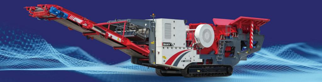
It is used for primary crushing and recycling of hard materials with compressive strength not exceeding 300Mpa in construction, transportation, railway, cement, building materials, metallurgy, tailings and other industries.
